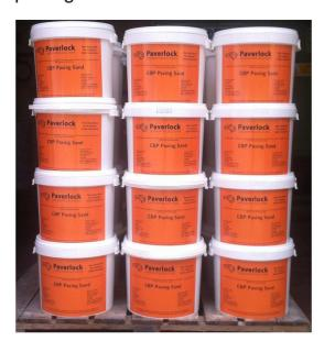
Paverlock Jointing Sand's unique formulation is based on a pre-blend of carefully selected sands and an organic additive, which is non-toxic, contains no cement or resins and reacts with atmospheric moisture to bind the sand into the joint, whilst still allowing flexibility, which is an important feature of interlocking paving systems.
